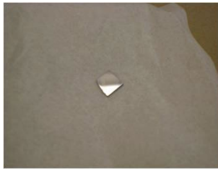
Figure XI: Ag/Si ( 7 \times 7 ) sample, showing evidence of silver deposition everywhere but at the corners (covered during deposition).
